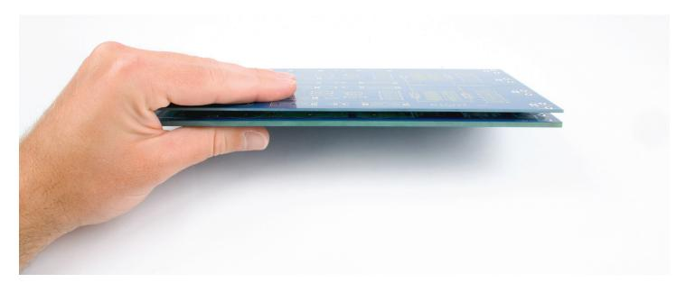
The Duos addresses the issue of circuit board dielectric by doubling the thickness of an FR4 fiberglass circuit board. Just that one choice reduces electric field strength by one-half. Additionally, the area of copper interacting with board dielectric is also reduced in critical regions. Signal lines are kept narrow. Power lines are extremely wide. Such choices get us refined performance. Good solid advantages based up the application of good solid physics.
